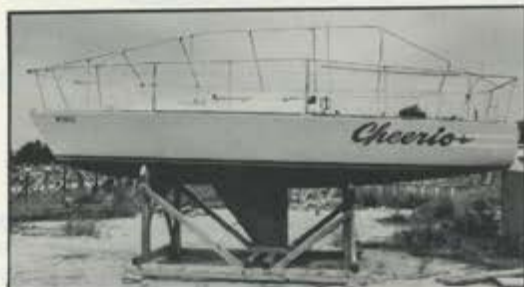
A J-24 with newly constructed frame. Using ordinary tools, the job takes about 3-4 hours to assemble, a half hour to disassemble. (Below) Form-fitting, treated cover provides the ultimate protection.
