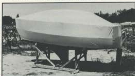
A J-24 with newly constructed frame. Using ordinary tools, the job takes about 3-4 hours to assemble, a half hour to disassemble. (Below) Form-fitting, treated cover provides the ultimate protection.
