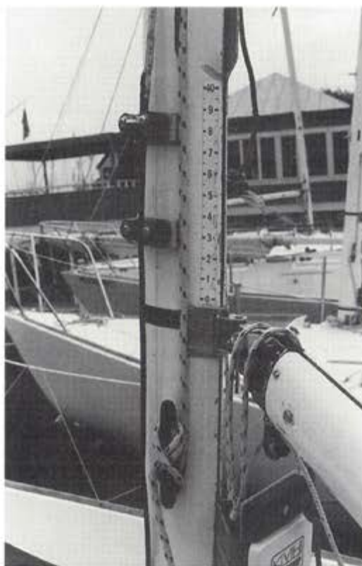
In addition to the mainsail cleat, this owner has elected to put the jib halyard cleats to port also.
