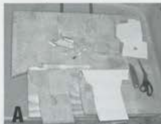
The pattern you create in cardboard (A) is transferred to the balsa core to assure a tight fit (B).
