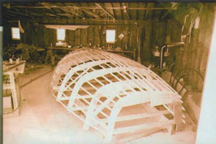
"Ragtime" wood hull form takes shape in the garage -Jan., 1975
