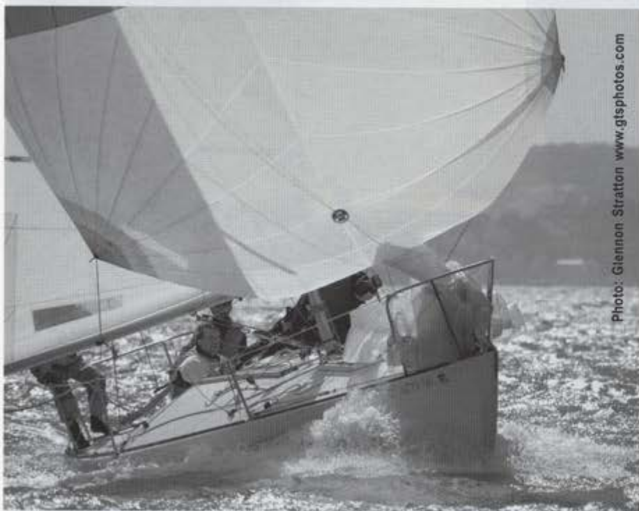
A loose leeward twing helps open the leech of the spinnaker when reaching in heavy air.
