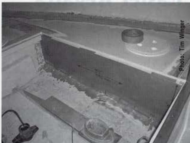
A cardboard template is created to pattern the new interior side panels. Note the inspection port is installed before the side panel.
