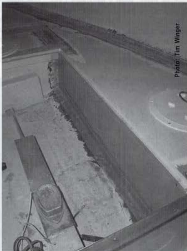
The completed side panel is installed and ready for painting.
