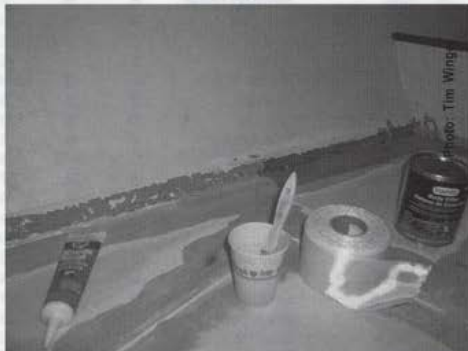
The edges are ground back to bare fiberglass and wood in preparation for sealing the new air tanks.
