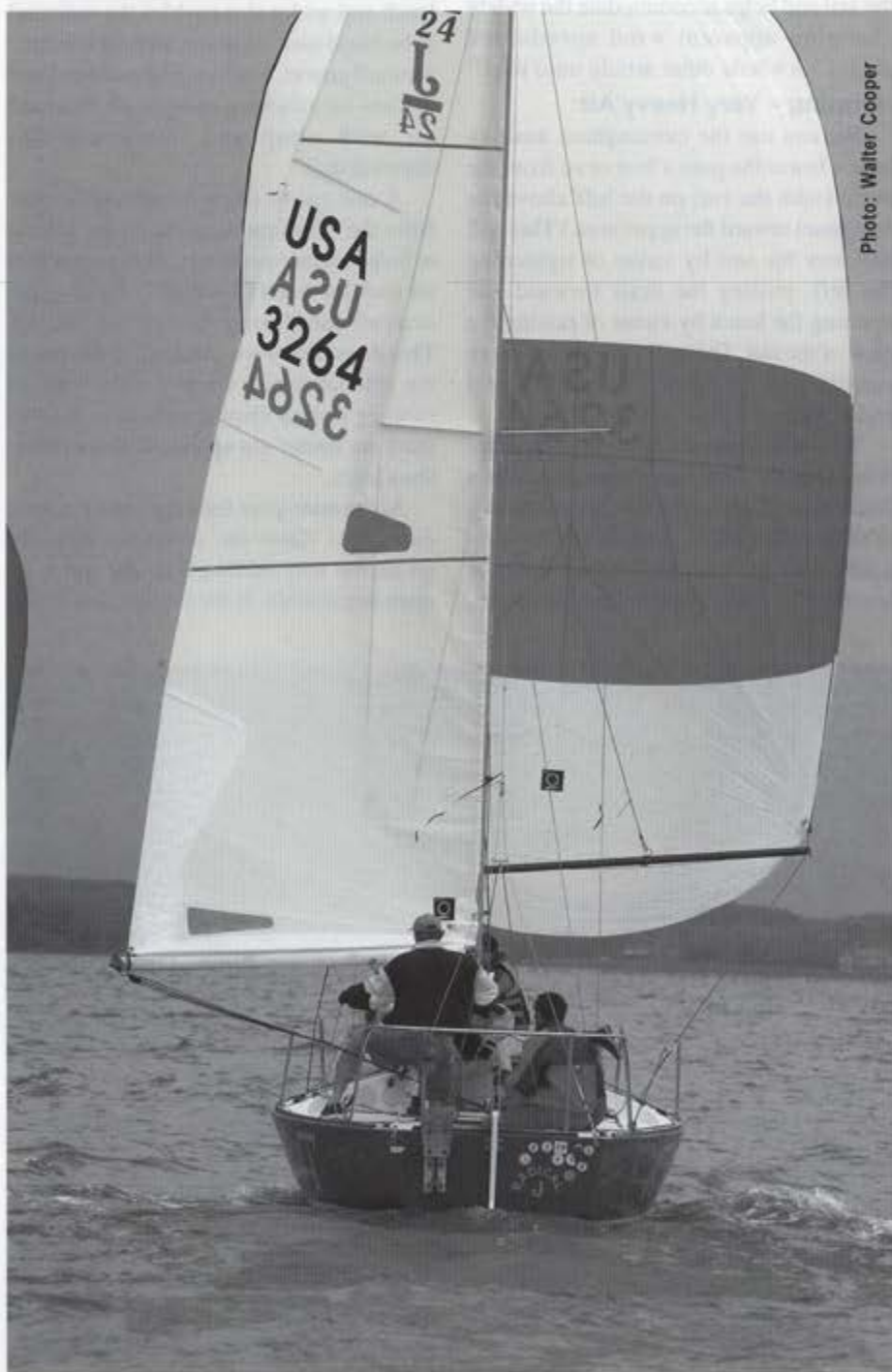
A level pole will help maximize the sail's projected area while running in medium air.
